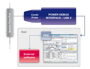
Fig. 26: CombiProbe can be configured so that external software can process trace information at recording time.
