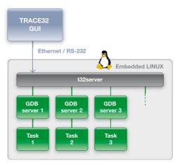
Fig. 1: The t32server service, enabling simultaneous debugging of two or more application processes
