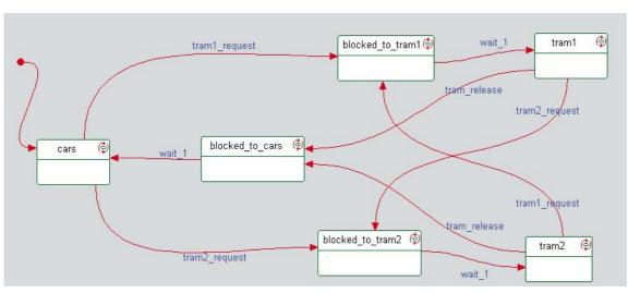
Fig. 7: State diagram of new traffic-light switching
