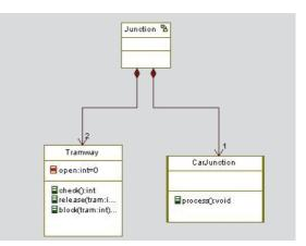
Fig. 6: The new class, "Junction", integrating the "old" traffic-light switching and the two new traffic lights for the tram
