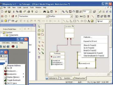
**Fig 8:** The integration of TRACE32 and Rhapsody allows a debugging in UML, C++ and C.
