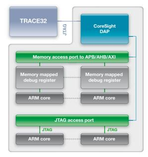
**Fig. 14:** The DAP can always address the debug logic of the individual cores directly. This means it is no longer possible for the switching off of a clock for an individual core to block debugging of the entire chip.
