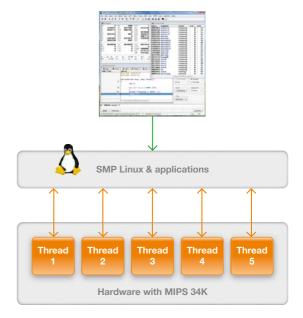
Fig. 19: Only one instance of the TRACE32 debugger is used for debugging all cores or hardware threads.
