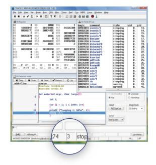
Fig. 21: The TRACE32 window, which always shows only the context of a core or hardware thread. The number of the core or hardware thread is shown in the status line.
