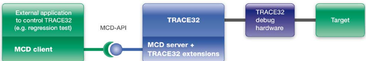
Fig. 17: TRACE32 can be controlled by an external application over its Remote API.
