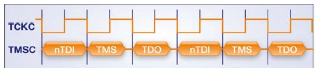
Fig. 16: Simplified diagram of the 1149.7 protocol
