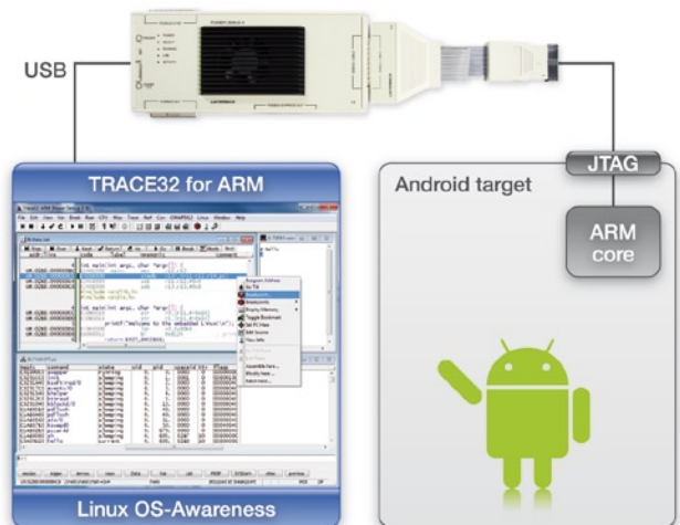
Fig. 4: In stop-mode debugging, the debugger communicates directly with the processor on the Android hardware platform.
