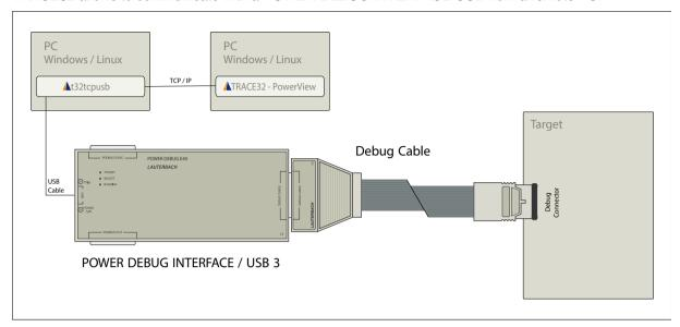
In order to implement this communication, the command line tool **t32tcpusb** has to be started on the PC to which the POWER DEBUG INTERFACE USB is connected. **t32tcpusb** can be found in the bin/<target\_os> directory of your TRACE32 installation (e.g. bin/windows64).
