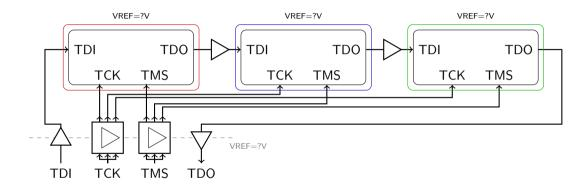
• In case of different I/O Voltages multiple level shifters are required
