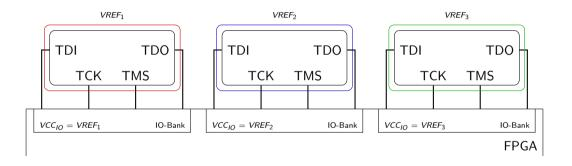
• IO-Banks of a (small) FPGA may be also used as level shifters
