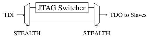
To support this feature, the circuitry of the JTAG Switcher is slightly modified like this:
