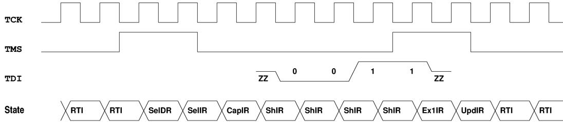
The JTAG TAP Controller state sequence starts in the *Run-Test/Idle* state. The IR code **1100** is shifted into the IR (least-significant first). After setting the IR code, it is now possible to set the bus address via a DR-Shift Sequence:
