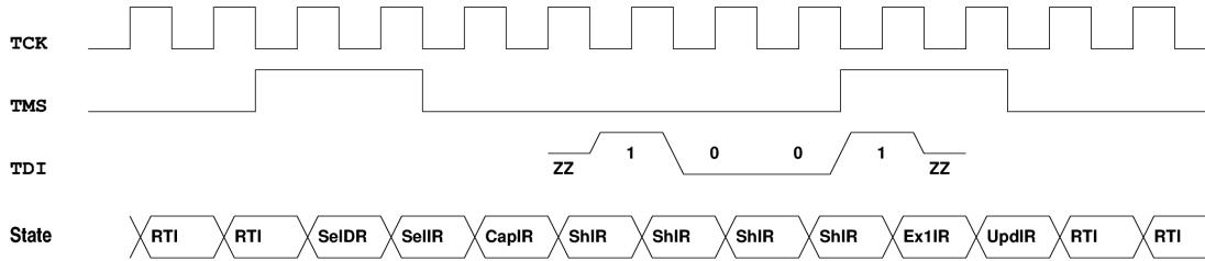
The IR code **1001** is shifted into the IR. After setting this IR code, it is now possible to write a 16-bit value to the specified bus address and bank:
