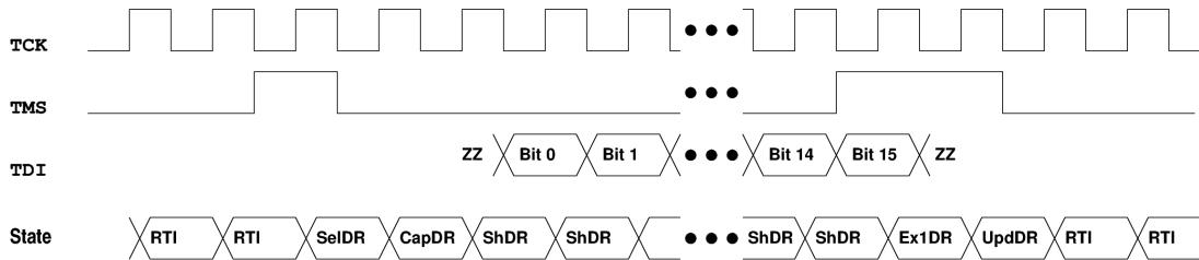
Bit  $2..0$  of the 16-bit value are used to set the address, bit  $15..12$  are used to set the bank. To execute a write access, you next have to set the IR to another value:
