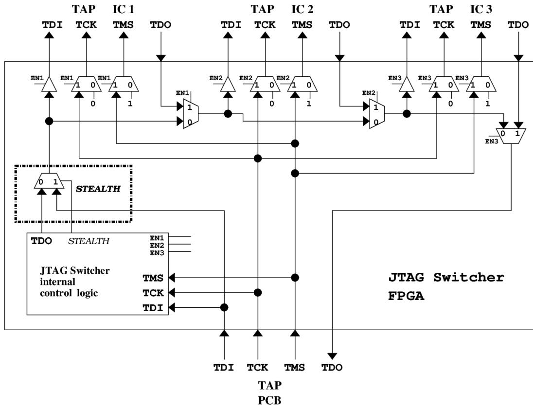
As depicted above: Once Stealth Mode is enabled, the TDI-TDO path of the JTAG Switcher TAP is bypassed. The effect is, that from the outside the JTAG Switcher TAP is not visible anymore.
