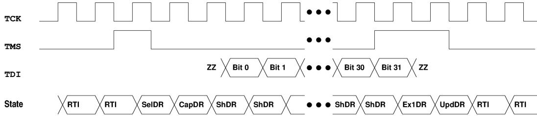
Here bits  $15..0$  define the 16-bit value to be written to the address specified by bits  $31..16$ .
