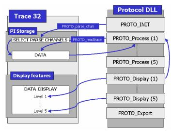
The library must be designed following few very specific rules: an initialization (**PROTO\_init**) selects and prepares the channels that must then be read by the API function
