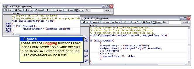
**T32\_KLoggerAddr** logs an *address*, in order to trace the transition to a specific point of the code, while **T32\_KLoggerData** aims to log *address and data* of any **write cycle** executed by the microprocessor; being called in appropriate points of the code, these two functions can achieve the desired task.
