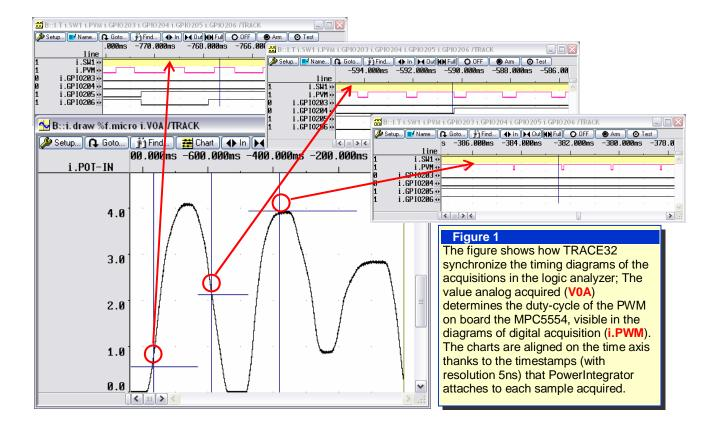
As the MPC5554 processor also includes a Nexus trace unit, we can record the real-time trace of the code. Through this mechanism it is easy to correlate events within the hardware to the specific software routines that generated them.
