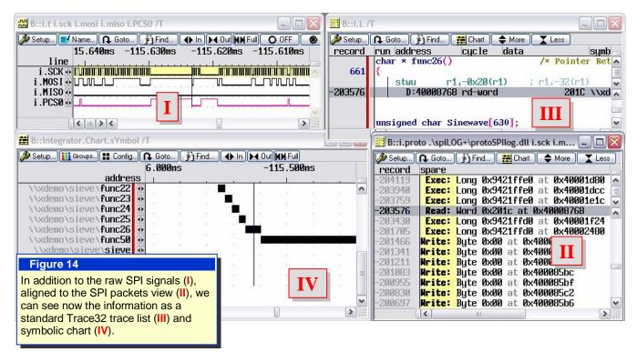
It is worth comparing what has been done in this example of data logging using **Protocol Analysis** as compared to the previous data from the **Bus trace**:
