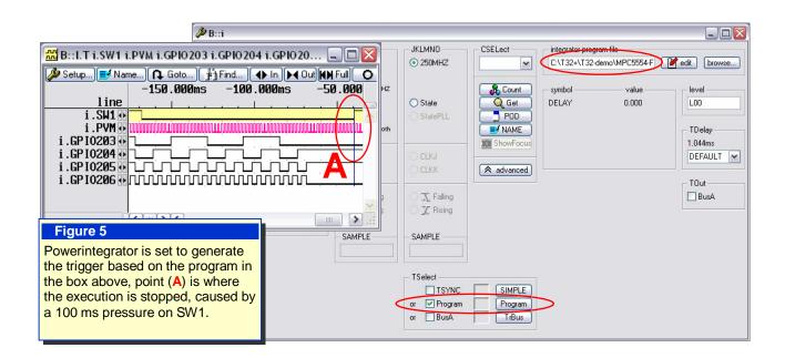
From this basis it is easy to understand how the PowerIntegrator can implement triggers controlled by very complex conditions. It can control the software execution based upon the behaviour of the hardware and the software.
