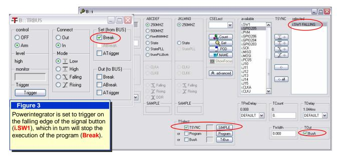
The visible effect is that when pressing the SW1 button on the board, the falling edge generated on the channel being monitored (i.SW1) stops the execution of the program.
