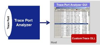
Figure 2: A *Custom Trace DLL* performs the task to analyze and display the payload within the trace port analyzer GUI when conventional tracing is used.
