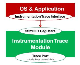
Figure 1: Instrumentation Trace with dedicated off-chip Trace Port
