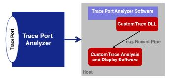
Figure 3: The *Custom Trace DLL* extracts the payload and passes it to the *Custom Trace Analysis and Display Software* when the trace port analyzer works in real-time streaming mode.
