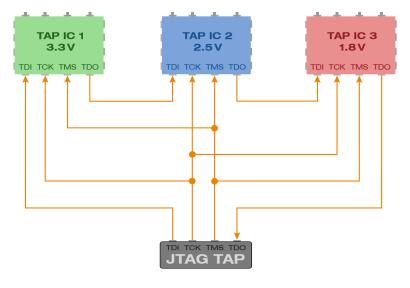
Figure 3: Different voltage levels require additional PCB design work
