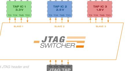
Figure 5: A JTAG Switcher placed between the board JTAG header and the individual devices allows a seamless debugging
