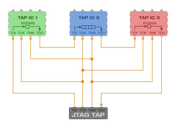
Figure 2: Bypassing TAP IC 1 and TAP IC 3 allows a debugger to communicate with TAP IC 2
