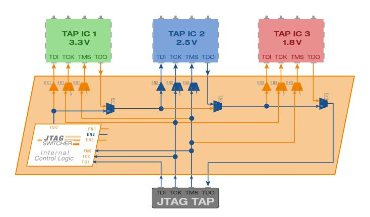
Figure 6: EN2 is active, this allows a debugger to communicate with TAP IC 2
