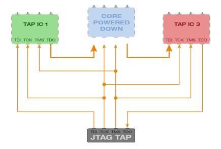
As embedded designs strive for even greater efficiency and prolonged battery life, devices are regularly put into low power or sleep modes when they are not currently active. An example can be seen in figure 4.
