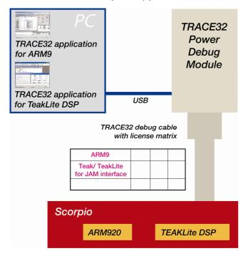
Fig. 1 Debugging ARM920 and TeakLite DSPs in Scorpio over a common TRACE32 ICD
