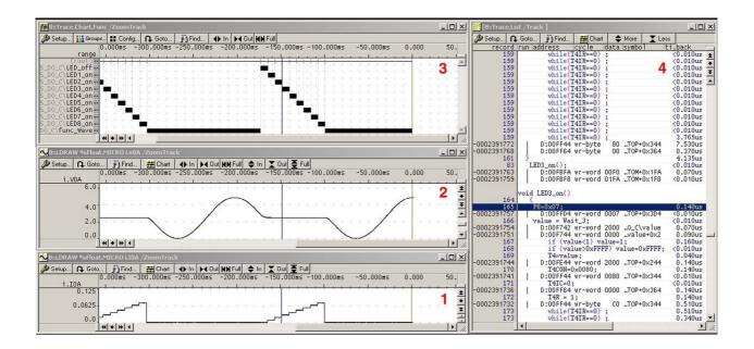
Statistical analyses are run automatically after each program stop. They provide information about mini-mum, maximum and mean values of the energy consumption of the executed functions. Similarly, the absolute and percentage share of the total energy consumption is calculated for each function. This makes it easy to locate the program parts that use the most energy.
